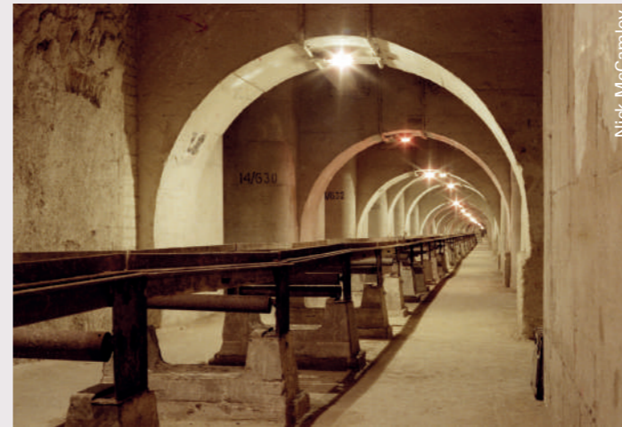
Conveyor belts transported ammunition within the mines.
